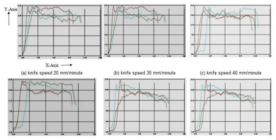
Figure 4. (a-c) and (d-f) Cutting force (Newton, Y-axis) vs. Depth of cut (millimetre, X-axis) for Potato cuboids of contact area (400 and 500 square millimetres respectively),\*Three individual colour lines in graph showing the 3 replicates for each experimental sample
